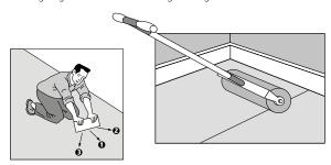
Joints do not require sealing by hot or cold welding.
