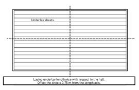
The length of the foam rolls allows to not have any butt or header joints in the gym.
