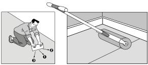
Fold back the sheets halfway to apply glue. Begin application with the central half-sheets on either side of the length axis. Fold back the second halves and proceed likewise, then apply to the neighbouring sheets edge to edge leaving a gap of 1 mm + or - 0.5 until reaching the walls.
